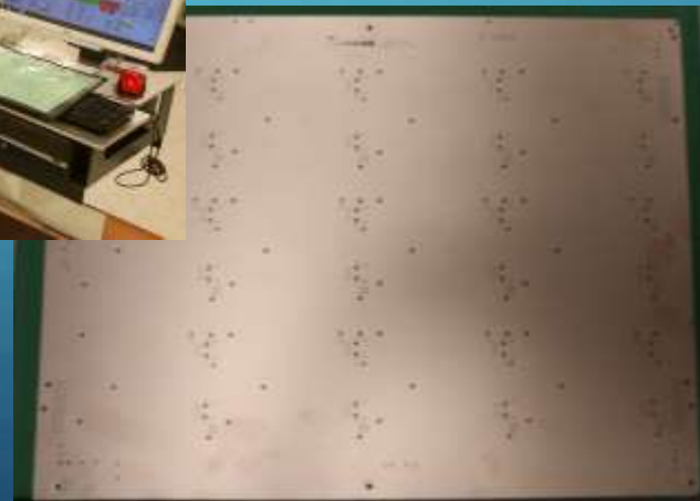
PANEL AFTER DRILLING
