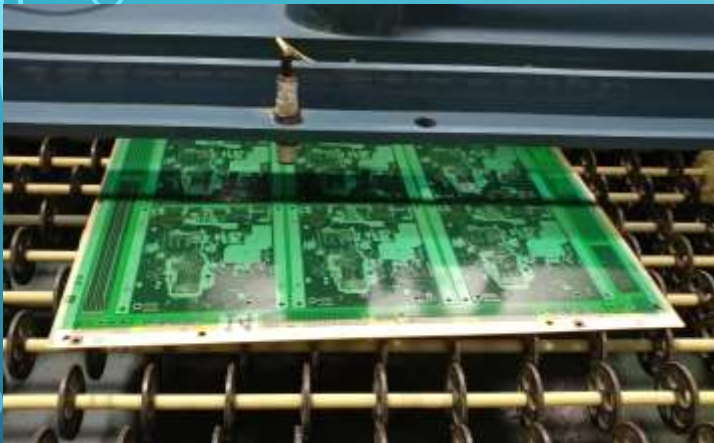
PANEL EXITING THE DEVELOPER, ONLY DESIRED SOLDER MASK LAYER REMAINING
