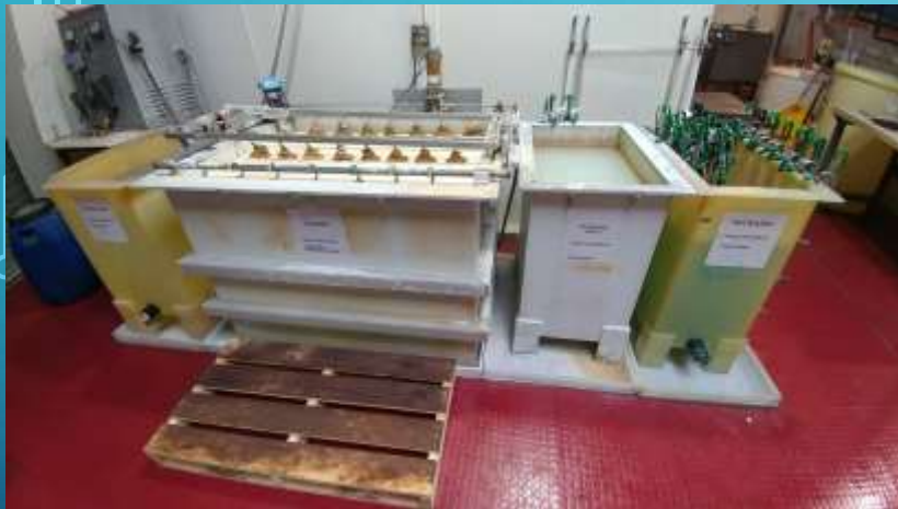
PANELS ARE PLACED INTO A TIN PLATING TANK
