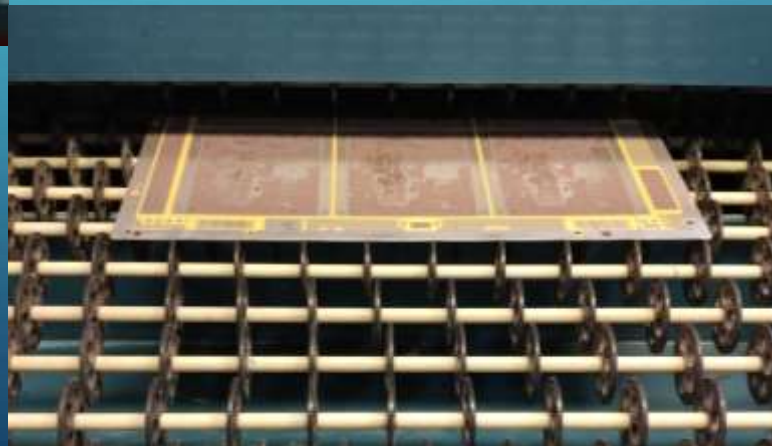
PANELS EXITING ETCHER – ALL UNPROTECTED COPPER ETCHED OFF
