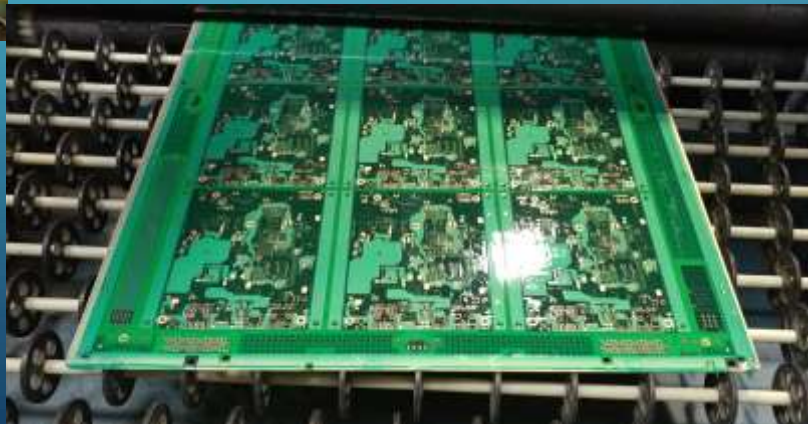
PANEL EXITING THE DEVELOPER, ONLY DESIRED SOLDER MASK LAYER REMAINING
