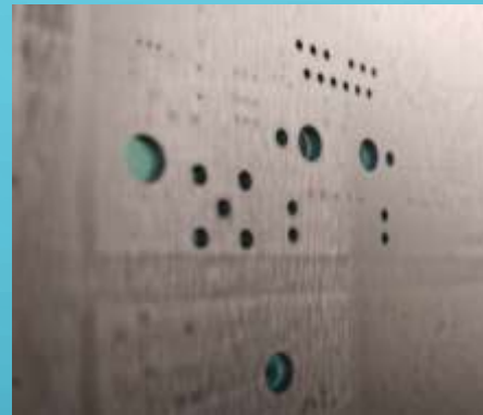
THROUGH HOLES BEFORE & AFTER ELECTROLESS
