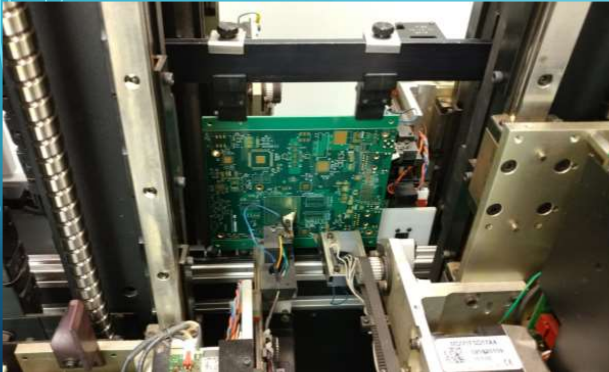
“FLYING PROBE” ELECTRICAL TEST
