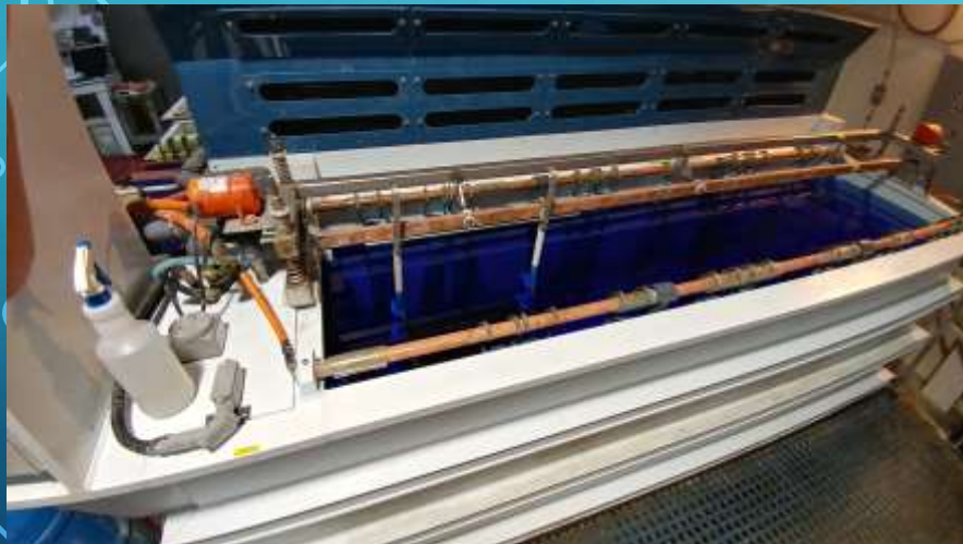
PANEL IN SECOND COPPER PLATING TANK
